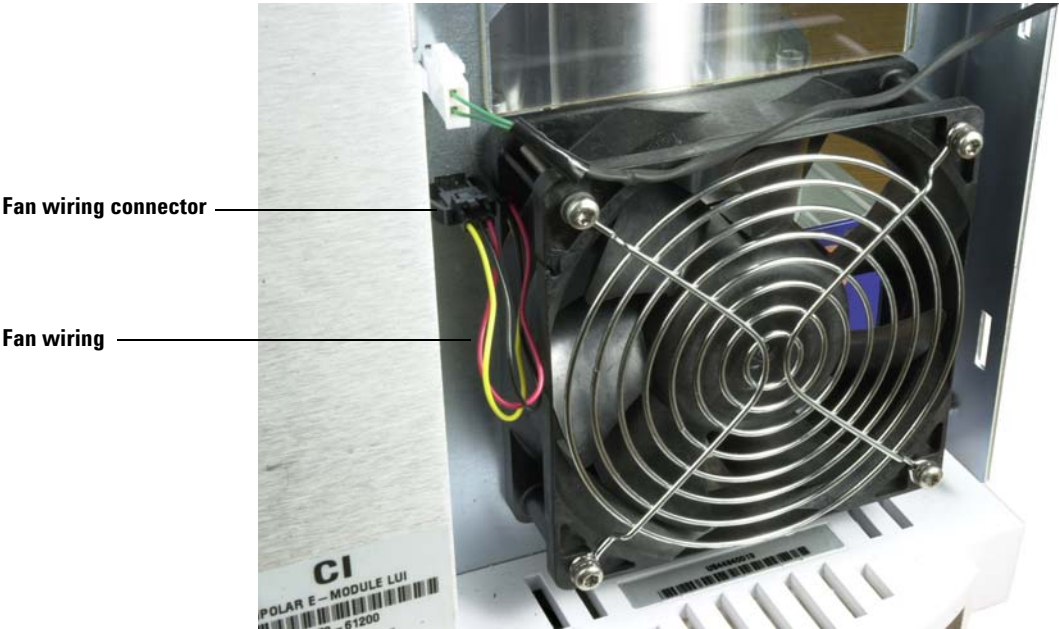
Figure 14 Replacing the pump fan (turbo pump shown)
