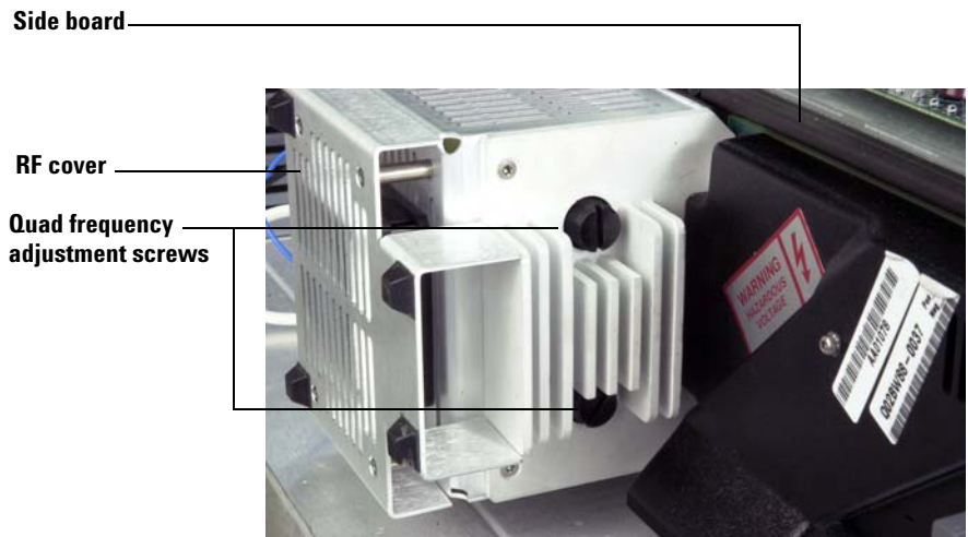
Figure 29 Adjusting the quad frequency
