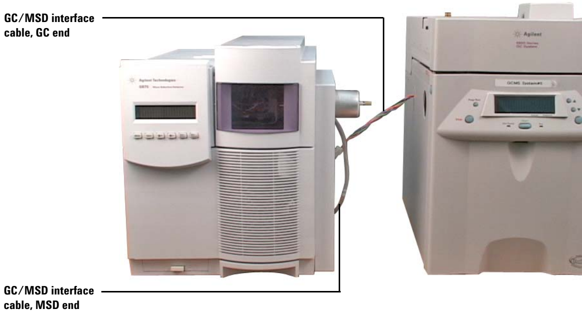
Figure 11 Interstitial panel installed, GC/MSD interface cable connected
