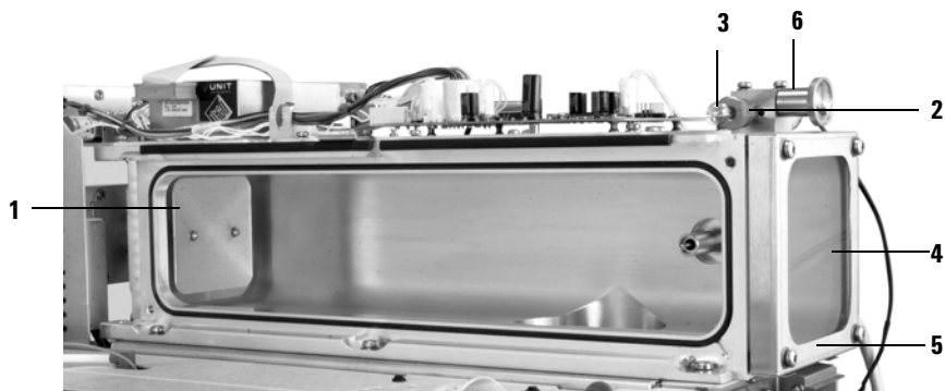
Figure 60 Analyzer chamber and related parts
